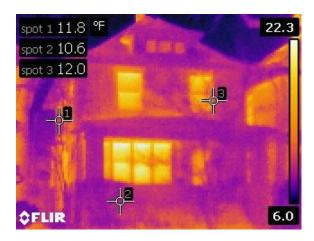
Figure 35: Thermal imaging data generated during a residential energy audit in Chicago, Illinois. Photo courtesy of Doug Farr, Farr Associates.
