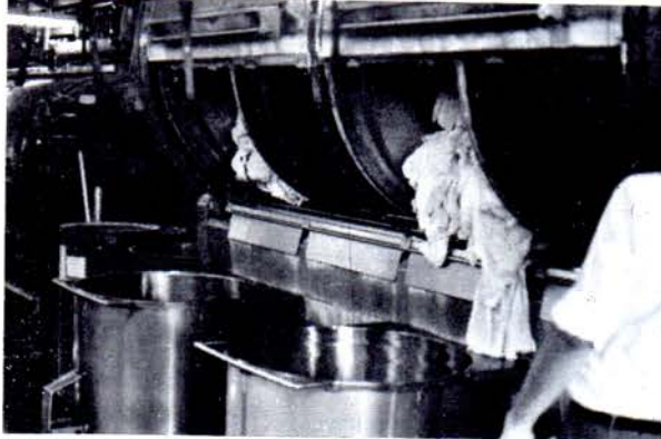
Mass production is the name of the game in the new ESH Laundry. Washers that stand taller than a man wash, rinse, and eject the clothes into the steel tubs (bottom center). The washers are loaded from the second floor through chutes. (ESH Photo)
