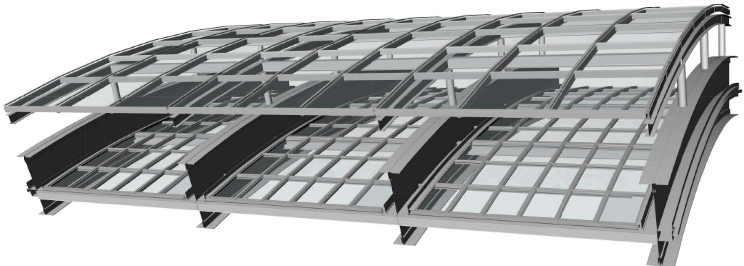
PROPOSED SKYLIGHT CONSTRUCTION RESTORATION OF HISTORIC SKYLIGHT (BOTTOM) NEW ENERGY EFFICIENT SKYLIGHT (TOP)
